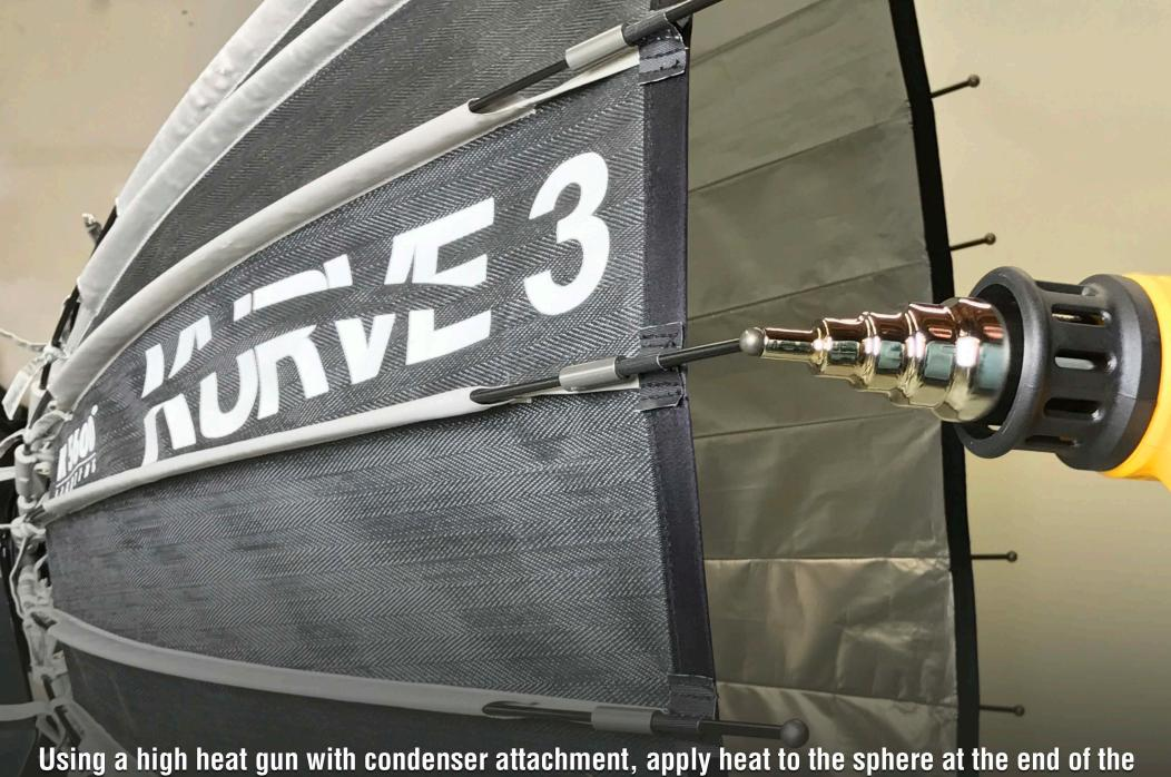
Using a high heat gun with condenser attachment, apply heat to the sphere at the end of the spoke. Heat will soften the glue used to hold the sphere at the end of the spoke. Be sure not to apply heat directly to the spoke as it will cause the spoke to enlarge and make it nearly impossible to remove from the umbrella without cutting.
