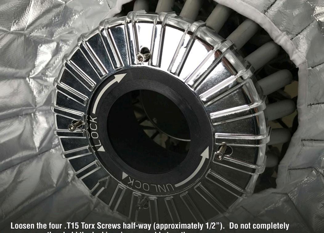
remove as they hold the locking ring assembly together.
