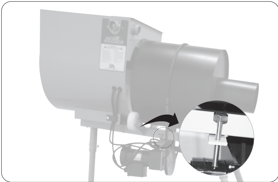
Figure 3 Insure sufficient tension on the tensioning bolt to keep the belt from slipping. To apply tension, rotate bolt clockwise.
