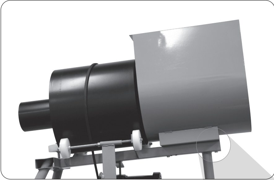
Figure 1 Bolt ball Reservoir to main frame, using washers and bolt.
