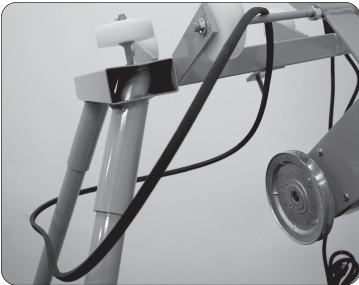
Figure 2 Place belt around main frame as shown for easier assembly to tumbler.
