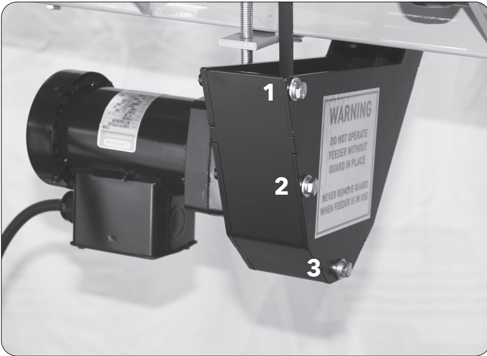
Figure 10a Install drive belt guard as shown
