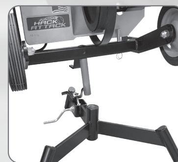
Figure 8D Lift the throwing head completely out of the undercarriage.
