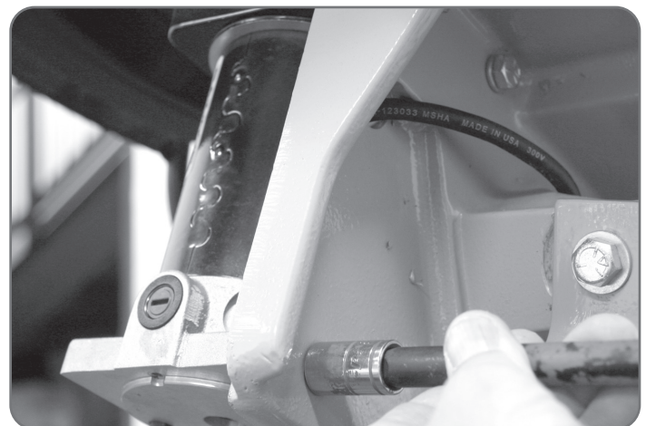
Figure 10 Shown using a 6" extension with 7/16" socket.
