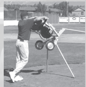
Figure 3 Begin to lift Junior Hack Attack upright (See Safety Hint at lower left).
