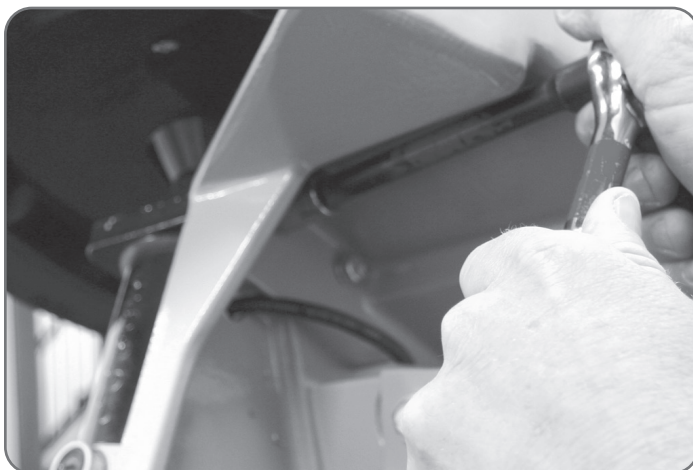
Figure 9 Shown using a 6" extension with 1/2" socket.
