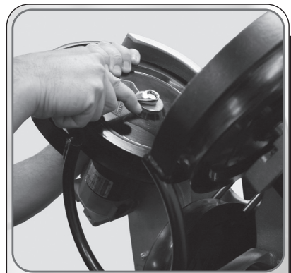
Hold wheel while loosening bolts.
