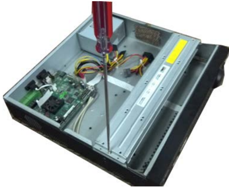
Figure 3-32 Open the top cover
