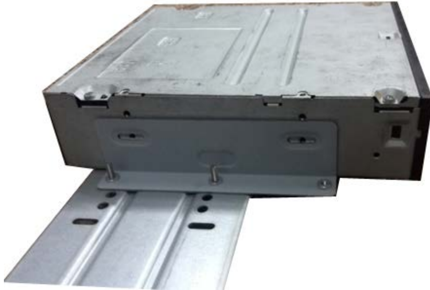
Figure 3-38 Install SATA burner
