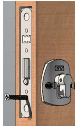
Fig 6 Fit the lock in the mortise. Do not use a hammer to force the case. Fit the lockguards, and internal pull if using, on either side of the door with the bolts provided. Next, fit the thumb turn cylinder in the lock case. Fit the cylinder screw through the lock case to fasten the cylinder.
