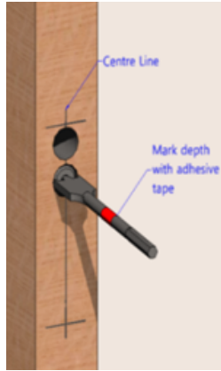
Fig 2 Mark a centre line* between the marked lock case lines. Drill a series of 19mm diameter holes a little deeper than the lock depth. Do not drill above or below lock case lines. *For doors more than 50mm thick, mark an offset line
