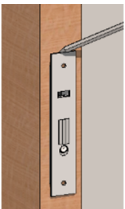
Fig 4 Insert the lock case and mark the cover plate outline. Chisel out a 4mm recess so the cover plate is flush with the door edge.
