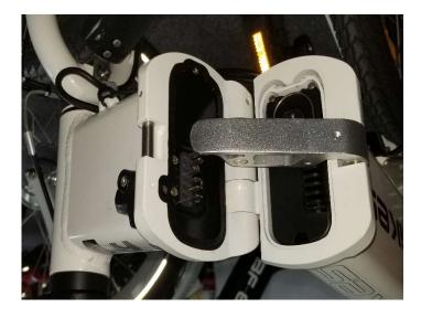
The lever can push against the battery pins which will bend the pins and prevent the frame from closing. **Operation of speed control:**
