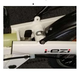
• Lift up safety catch on the centre frame clamp
