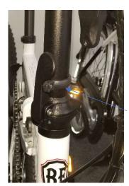
Steering stem safety ring engaged into locking lever
