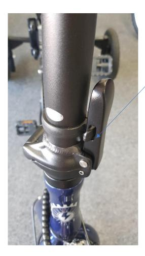
Steering stem safety ring engaged into locking lever (tongue ring must protrude through hole in mechanism)
