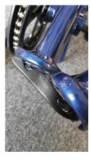
The lever can push against the battery pins which will bend the pins and prevent the frame from closing.
