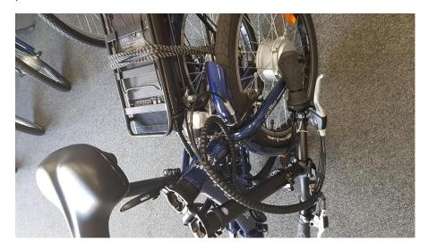
**Note:** When unfolding the BF ezi-Step make sure that the frame lever is **not** closed into towards the frame as shown in the photo. as shown in the photo. Always ensure the lever is hinged out, away from the frame.
