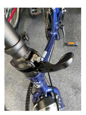
• Fold the head stem clamp at base of the handlebar stem and allow the handlebars to lay down, being careful to tuck the cable to the inside towards bike frame so it does not bow outwards and secure with bungy strap
