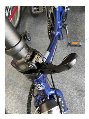
Steering stem safety ring open and unlocked
