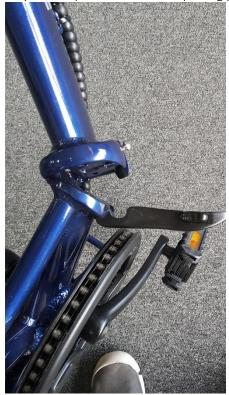
• The front wheel will fold around towards the rear of the bike like a clam shell. Continue the fold all the way back keeping the front wheel straight so front wheel meets rear wheel
