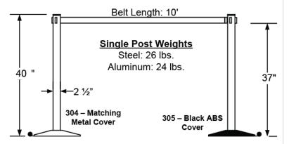
Specs for 10' Single Line Retracta-Belt with Retracta-Wheel Base (other models available)
