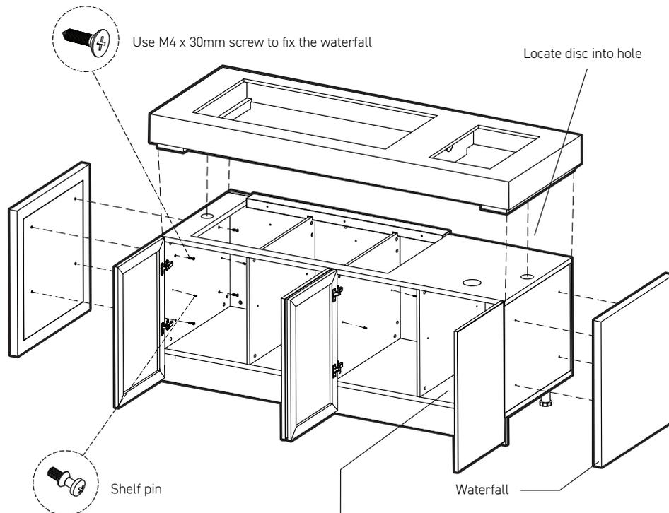
When assembling the waterfalls to the cabinet, the top of the waterfall must be level with the top of the cabinet, and there must be clearance between the bottom of the waterfall and the ground, adjust the leveling legs as required.
