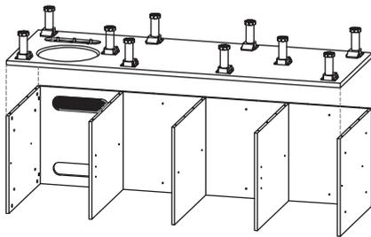
**5 Level the cabinet by adjusting the feet**
