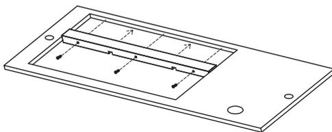
Use M4 x 30mm screws to fix the heat-resistant shield
