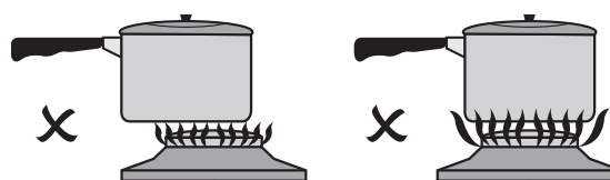
Incorrect - pan not centred.
