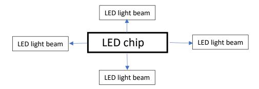
The semiconductor laser beam is a point light-source and can be collimated. The LED is a dispersed light source emitting at random times in random directions and needing a complicated optical system to have the light beam collimated. It is impossible to fully collimate an LED light source into the form-factor needed by a dental curing light.
