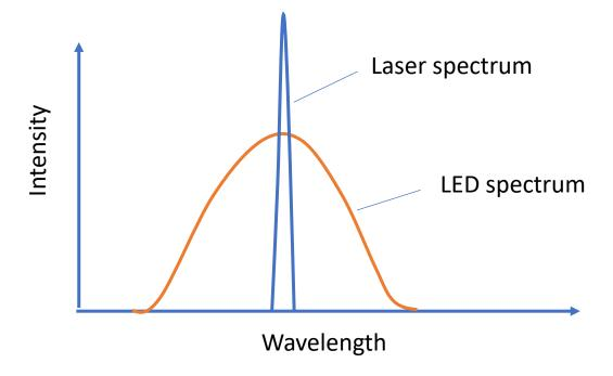
The narrow wavelength of a laser beam with its coherent behavior allows it to travel over long distances without a dramatic decrease in light intensity.
