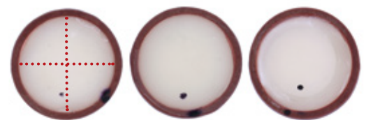
Width of cure samples in 20 mm molds. Hardness was measured at 1 mm intervals in the pattern shown. The area visibly affected by the light was always much larger than the actual cured material.
