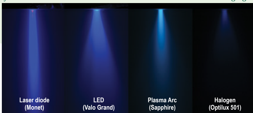
Beam comparison of four curing lights: The Monet laser exhibited an intense collimated beam while other light sources had greater beam divergence and diminishing energy.
