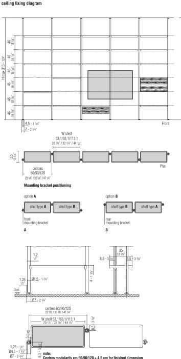
Centres modularity cm 60/90/120 + 4,5 cm for finished dimension (lower and upper feet protrusion cm 1,25)
