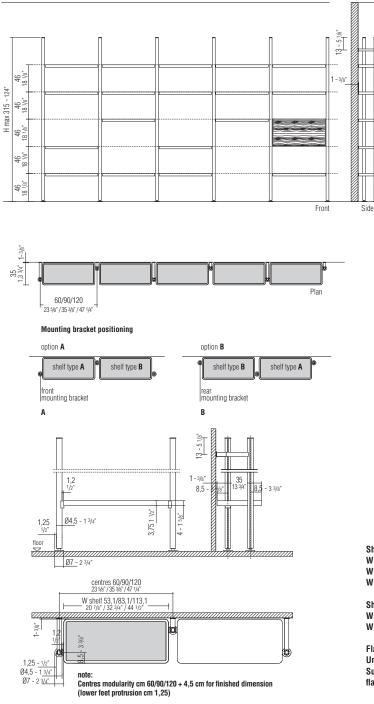
Shelf capacity with aluminium frame: W 53,1 = Kg. 15 W 83,1 = Kg. 23 W 113,1 = Kg. 27
