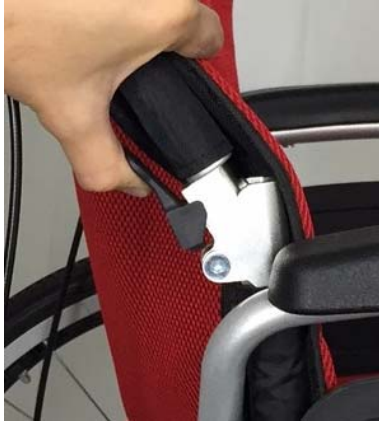
Push lever to fold back.
