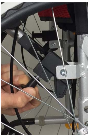
Pull back button to remove armrest.
