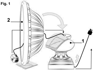
3. With the cord strung through both bowl and pedestal, lift the bowl on top of the pedestal while cautioning not to pinch the pumps power cord between both bowl and pedestal. Do this by removing the slack on the power cord. Once in place level the bowl using a beam level and shims or wobble wedges AG-16 available in clear, black and brown (not included).
