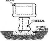
becoming unstable we suggest a solid stone block or pavestone whenever a pedestal is placed on a soft surface like dirt or grass.
