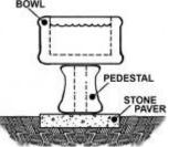
becoming unstable we suggest a solid stone block or pavestone whenever a pedestal is placed on a soft surface like dirt or grass.
