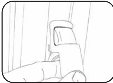
Unclip plastic cover on seatbelt slide.
