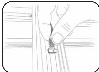
Slide bolts provided into roof rack.
