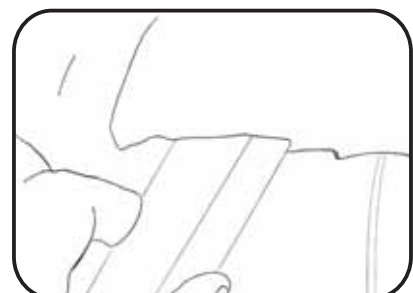
Gently pry plastic panels away from bodywork.
