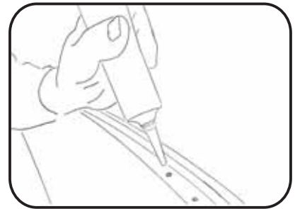
Silicone holes in roof.
