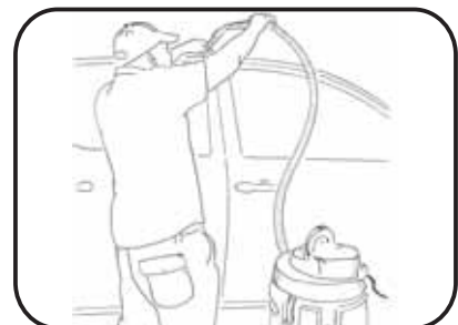
Remove aluminium track and vacuum groove.
