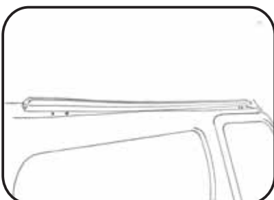
The K9 track will curve upwards once placed.
