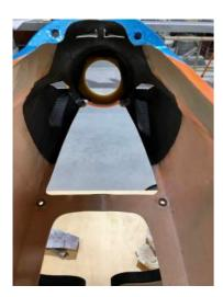
The included drill jig is aligned to the nose ring and taped in position with masking tape. A level can be used to help align the jig as shown. Drill one M4 hole and then fit an M4 screw and nut to hold the jig firmly. Repeat for the remaining three holes.
