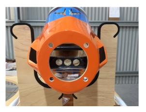
Remove the drill jig. Then open the holes out to 7mm that will allow the jig standoffs to pass through and later the included M4  $\times$  8mm CAP Head mounting screws.
