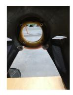
When trimmed correctly, the firewall should sit flat on all four standoffs and not foul with the fuse sides. Take your time here to get a neat fit. Once happy with the fit, glue the firewall into position with a quality 30 minute epoxy. We use Pacer brand 30 minute epoxy resin. The firewall is held in place by four M4 screws whilst the epoxy cures. As an option, you can run some 12k carbon tow around the circumference of the firewall for extra strength.
