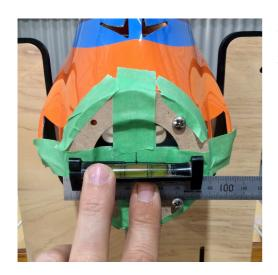
The included drill jig is aligned to the nose ring and taped in position with masking tape. A level can be used to help align the jig as shown. Drill one M4 hole and then fit an M4 screw and nut to hold the jig firmly. Repeat for the remaining three holes.
