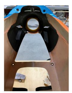
We strongly suggest laminating the inside of your fuselage nose with light weight (120-150g/sqm) carbon cloth. This will improve the strength and rigidity of the nose area. Some models come with carbon in the nose already.
