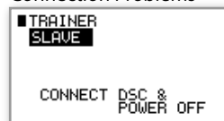
The cable is not connected or the power is switched on.
