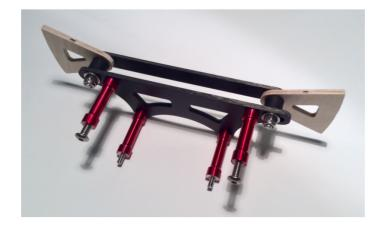
9. Firstly, remove the top two M3 x 8mm screws from the top of your Adverrun Single Drive. The M3 Cone washers will be reused so set them aside for the moment.
