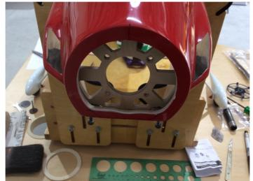
7. You can now test fit the Adverrun Single Drive to the fuselage using the M4 x 8mm screws. Replace the Adverrun supplied 5mm prop hub spacer with the 7mm one provided in this kit. If all has gone well, the spinner should be nicely centred to the fuse nose ring. You should also have a uniform spinner to nose ring gap. The gap should be approximately 2-3mm.
