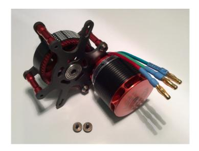
10. Next take the carbon rear support, M4 Nylon Nuts, M4 Flat washers and 10 x 8mm Rubber isolators and assemble them as shown.
