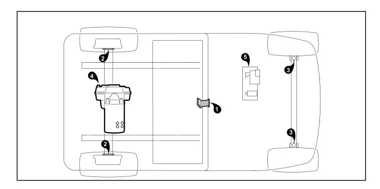
Figure 25 Lubrication Points – Electric Vehicles
