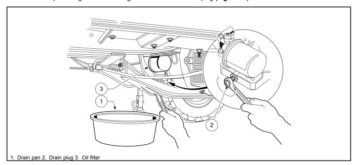
Figure 37 Engine Oil Drain Plug and Pan
