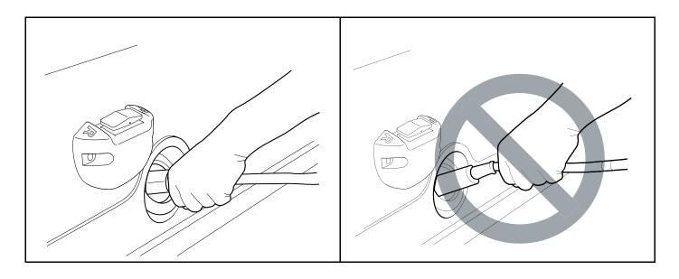
66 Figure 28 Correct Insertion of Charger DC Plug
