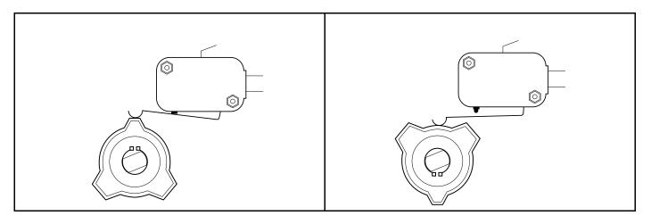
Figure 19 Neutral Lockout - Maintenance Position
