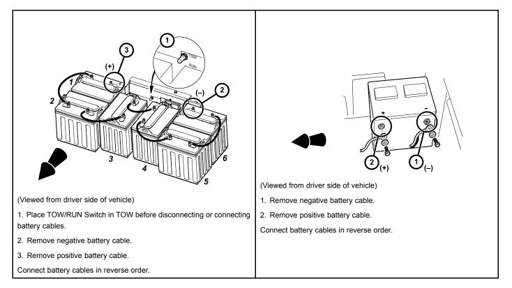
Figure 2 Battery Cable Removal – 6x8-Volt Battery Configuration
