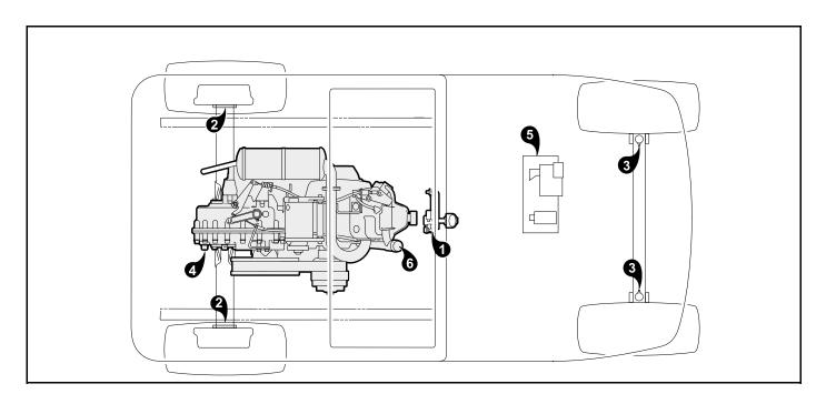
Figure 26 Lubrication Points – Gasoline Vehicles
