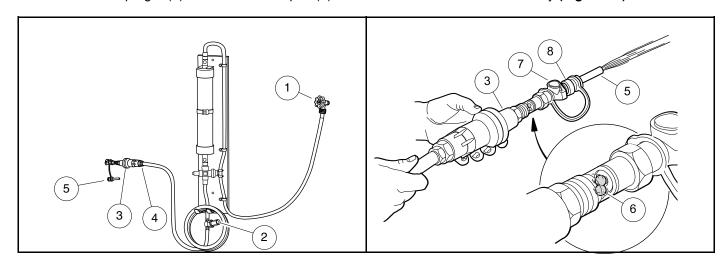
Figure 30 Connecting Hose with Filter to Water Source
