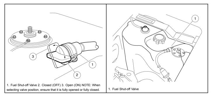
Figure 23 Fuel Shut-off Valve
