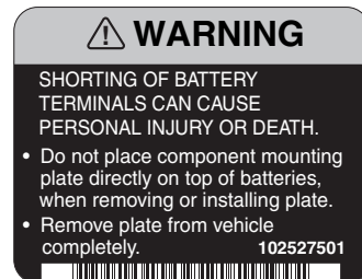
BATTERY TERMINAL WARNING DECAL (ON ELECTRICAL COMPONENT MOUNTING PLATE)
