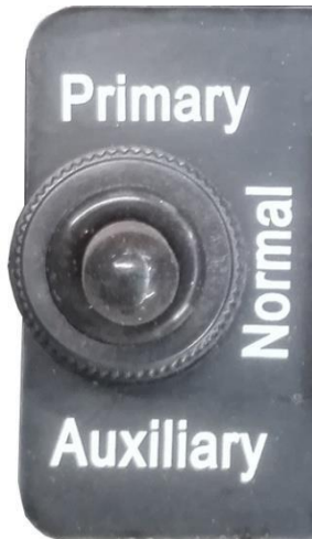
Figure 1: Parking brake switch in the middle position.
