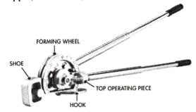
With this tool, bends can be made to any angle up to a full  $180^{\circ}$  return bend.
