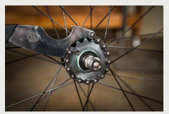
**e.** Use your chain whip and turn the fixed cog counter-clockwise to remove it. Set aside.
