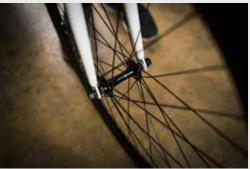
**c.** Finally, being mindful that the wheel is centered between the fork, tighten the axle nuts with your 15mm wrench.
