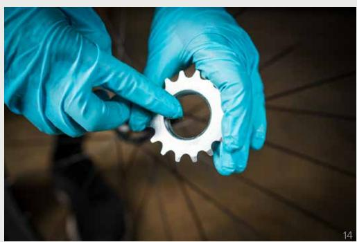
**g.** Install the cog by turning it clockwise. Tighten with your chain whip until you reach a hard stop.
