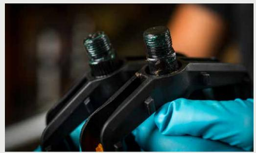
**c.** Finally, lightly grease the pedal threads.
