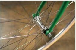
**c.** Grab your 15mm wrench and evenly tighten the nuts on the front wheel (make sure the wheel is centered between the fork).
