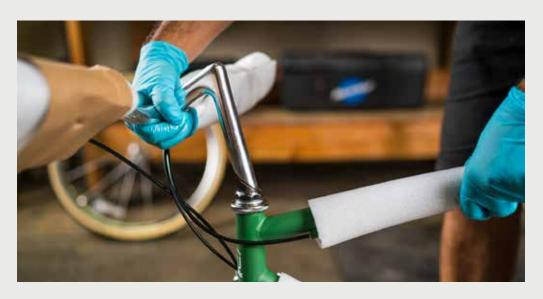
**d.** Finally, take your 6mm Allen Key and lightly tighten the bolt on the top of the qull stem into place (we'll fully tighten the quill stem a bit later).
