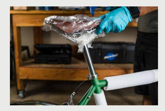
**d.** Finally, tighten the seatpost clamp with your 5mm Allen Key, making sure the saddle is centered/parallel to the top tube.
