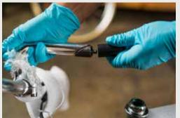
**c.** Now install the quill stem into the headtube, making sure the handlebars are facing forward *(away from the bike)*.
