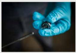
**c.** Slide the quick release into the hub from the left side.
