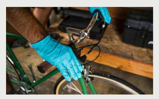
**b.** When you are balanced, place your hands on the handlebars and gently rotate the bars to your desired angle.
