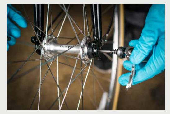
**d.** Reinsert the spring and screw the end cap back on.
