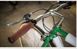
**b.** Now, stand over your bike and using your 6mm Allen Key, loosen the stem's top bolt.
