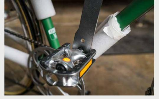
e. Repeat the same process for the left pedal, this time turning your spindle in a COUNTERCLOCKWISE motion instead. (note: left hand pedal has reverse threads)
