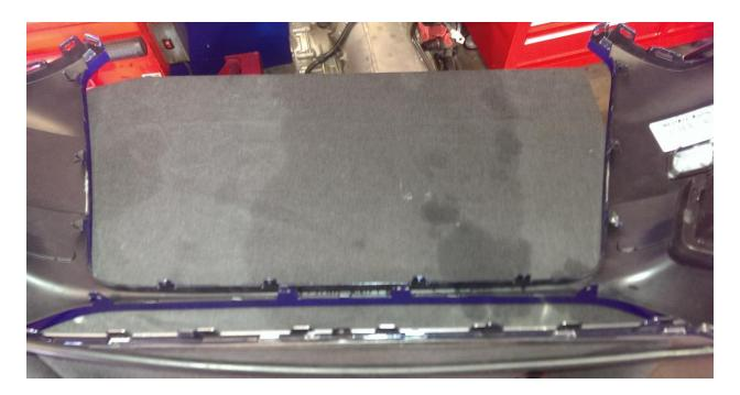
5. Installation is the reverse of removal, and the new grille will snap into the same tabs. There are also clips to mount the washer line. For those with park distance sensors, we recommend installing and starting the car before you bolt down the front bumper to ensure that the sensors are mounted properly so as not to cause false reads. Some users have reported removing the o-ring on the sensor to allow it to seat further into the grille.
