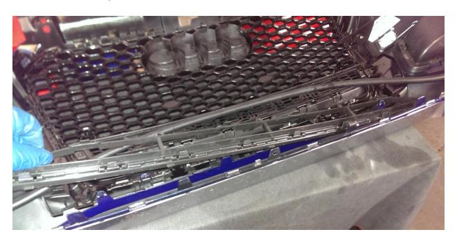
4. You are now ready to remove the OEM grille. There are 6 T25 screws holding the OEM grille in (3 on either side). Remove these, then gently unsnap the grille from the bumper. We recommend unsnapping the bottom portion, then moving to each of the sides. It should look like the following picture when you are finished. Use this picture for reference when unsnapping the tabs.
