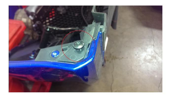
3. With this piece removed, you will now remove the lower air dam. First remove the phillips screws holding it in, then gently unsnap the piece from the bumper. These screws will not be re-used on the new grille, so store them somewhere safe.
