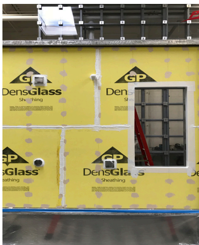
ASTM 2357 Test Panel - Detailing
