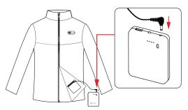
2 Select one or both zones. **Press and hold each button** for **3 seconds** to turn on or off.
