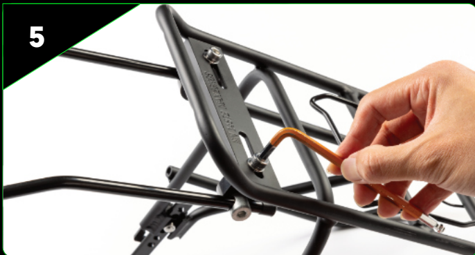
5 Attache forward mounting bars to Rear Pannier Rack using parts 8,15.
