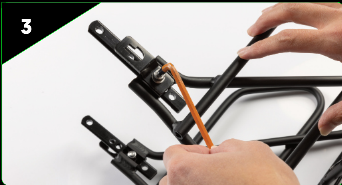
3 Attach Adjustable side mounting bars to the Rear Pannier Rack using the parts 10,7,12,11,14) leaving the single hole for mounting to the bike frame.
