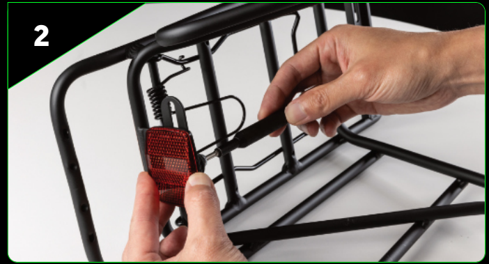
2 Re-attach Rear Reflector to the dedicated mounting plate o the Rear Pannier Rack.
