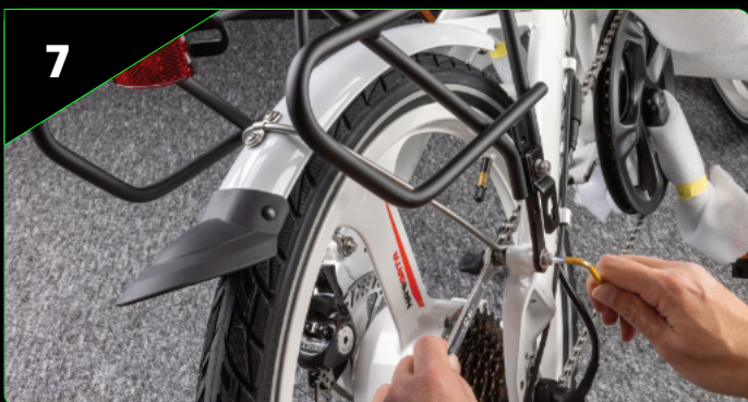
7 Attach side mounting bars with parts 6,14 the rear lower frame (chain stay)
