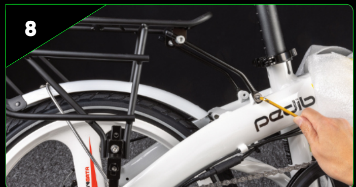
8 Attache the front mounting bar(s) to the frame using parts 9,14 (seat stay) & Now Rear Pannier Rack is fitted tighten all the nuts to complete assembly.
