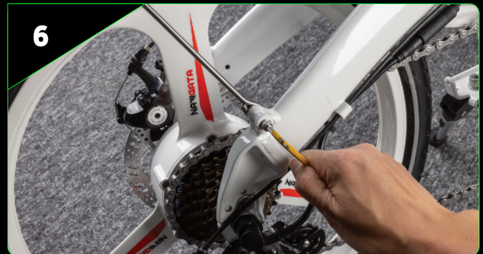
6 Remove the M4 34mm Allen socket cap bolt x2
