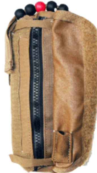
7.10 Continue zipping closed, slide fastener will separate. Mate zipper hook and loop tape.
