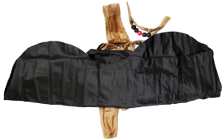
7.2 Fold bladder over so inflator is underneath then fold bladder in half, even with CO2 bottle (underneath)
