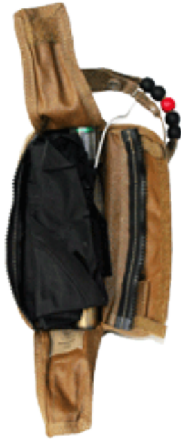
7.6 Fan fold other side of bladder on top of rolled portion and CO2.
