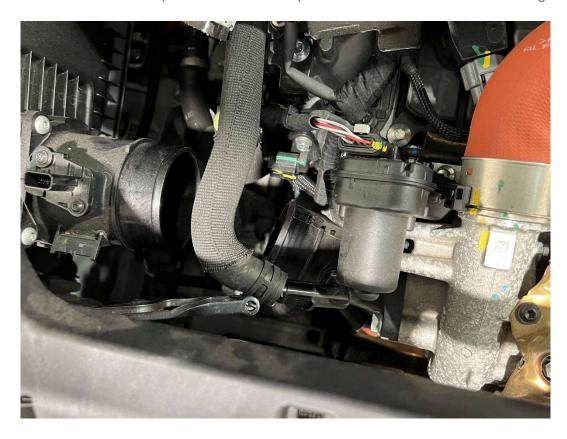
9. Remove the two 13mm bolts holding the standard inlet to the turbo. Be careful not to drop them!
