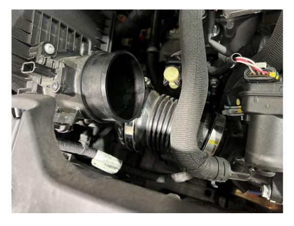
8. Remove the flexi portion and unclamp the two hoses from the remaining inlet.
