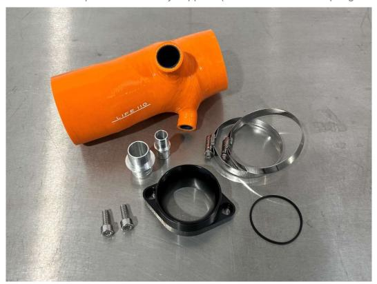
3. Prepare the hose by pushing in the aluminium connectors and positioning the clamps.
