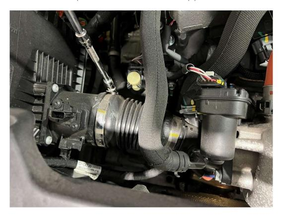
7. Pull up the end of the airbox away from its rubber mounts and the flexi pipe.
