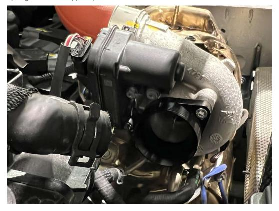
12. Put the new intake hose into place with the end connected to the turbo but do not clamp.
