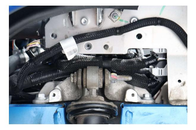
12. Now remove the rear spring damper modules from both the left and right sides of the car by removing the upper and lower bolts.
