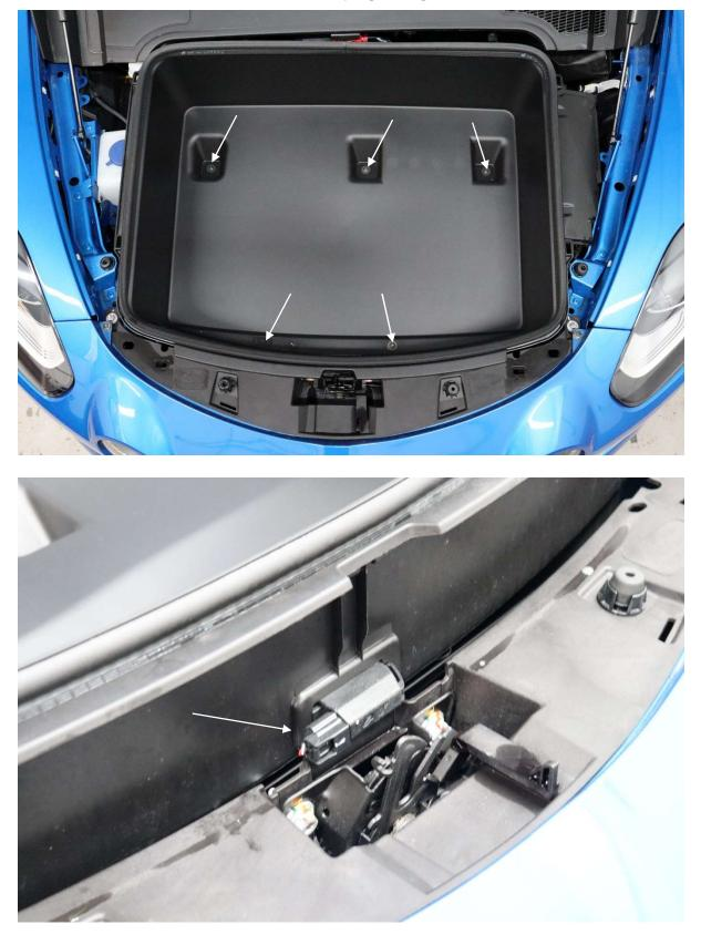
3. Unbolt the washer bottle and fuse box and move to one side.
