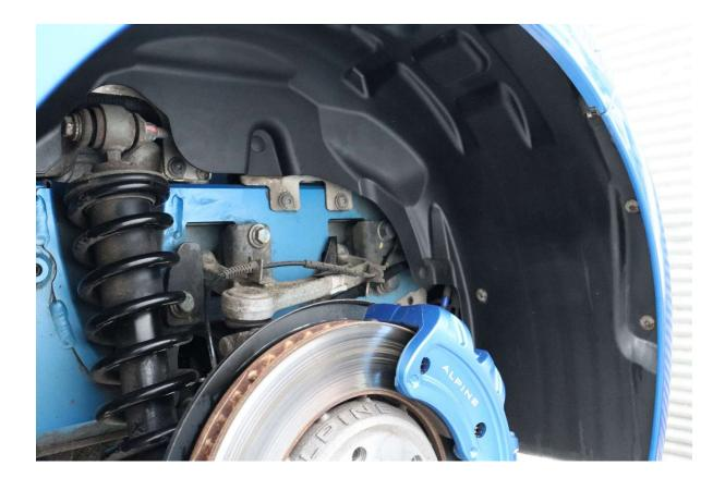
11. Remove the three torx head bolts from the bracket and unclip the wire to remove the bracket from the car.
