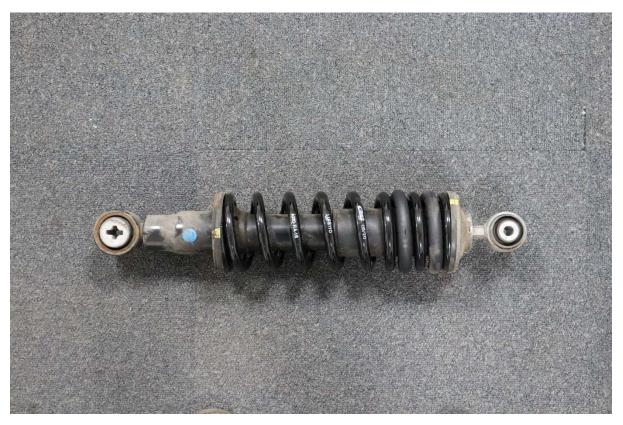
15. Refitting is a reversal of the removal process. Take note of the following care point: to ensure correct ride height tighten and torque the damper upper bolts to 105Nm with the wheels hanging into rebound.
