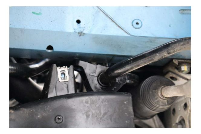
8. Remove the lower damper bolt from both sides of the front suspension.
