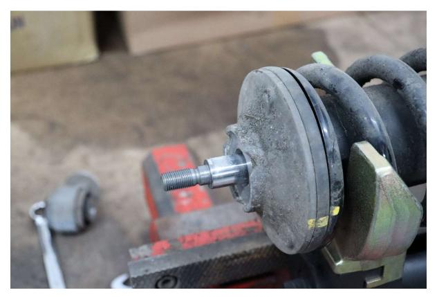
14. Replace the standard spring with the LIFE110 spring, ensure the spring is in the correct orientation. FA - front, RA - rear. Bolt the top mount back on with the upper and lower bolt holes in line.
