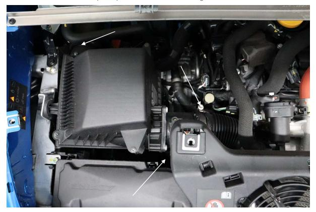
5. Remove the two torx bolts on the bracket revealed to the side of the airbox.
