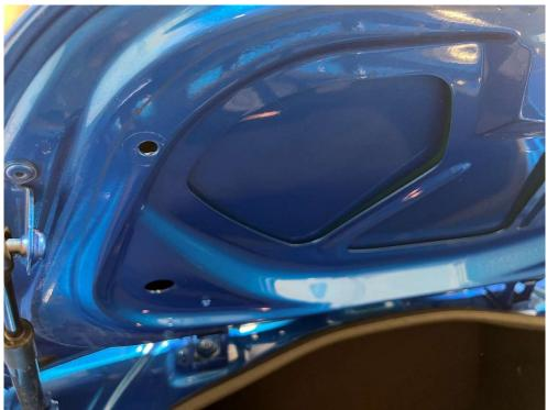
5. Push the supplied sandwich inserts between the upper and lower bootlid skins on both sides. These stiffen the structure once tightened to ensure the bootlid surface does not flex.
