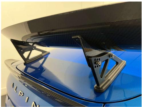
9. With the wing now firmly secured to the car fit the two endplates with the provided countersunk bolts.
