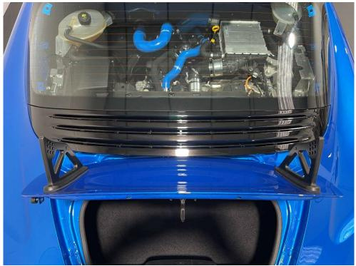
8. Now bolt the wing to the uprights. The wing will sit to the inside of the uprights and the bolts through from the outside of the car. Choose your desired position, the 'normal' position is the middle hole. Once the wing bolts are tight then fully tighten the upright bolts through the bootlid.
