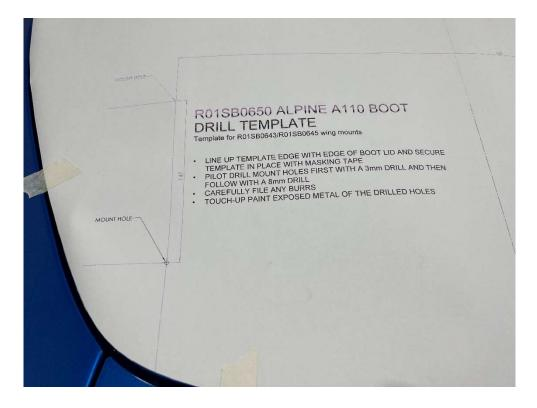
4. Drill the 4 holes to 8mm. We suggest using a 3mm pilot drill first then a step drill to achieve a neat 8mm hole. The rear most hole will pass through both upper and lower bootlid surfaces. You may wish to paint or primer the exposed metal.
