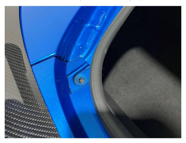
11. Assemble the bump stops as shown and screw into the vacant thread of the bumper fixing. You will need to adjust the height of these to get a perfect fit (use the position of the double nut locked together), the aim is for the bootlid to have a firm shut but not need to be slammed.
