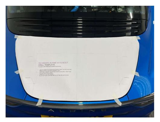
3. Use the template to mark through the hole positions onto the bootlid.
