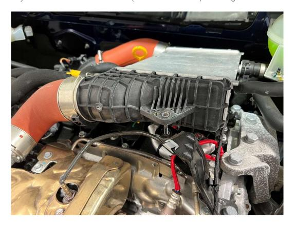
5. Use a screwdriver to open the front hose connector wire spring such that it can be disconnected from the intercooler.
