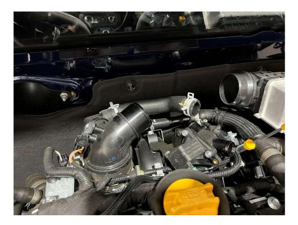
10. All hoses should now be removed. At this stage also remove the sound pipe link to the bulkhead (not shown in this example).
