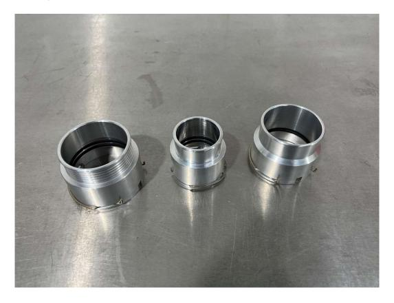
17. Apply a small amount of grease to the o-rings and then fit the three connectors to the intercooler and turbo, ensuring the wire springs clip into place.
