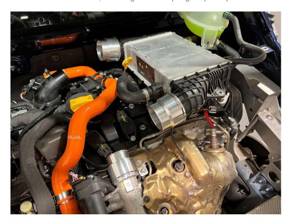
18. Fit the new front and back hoses and move the intercooler back onto its studs so everything is in place.
