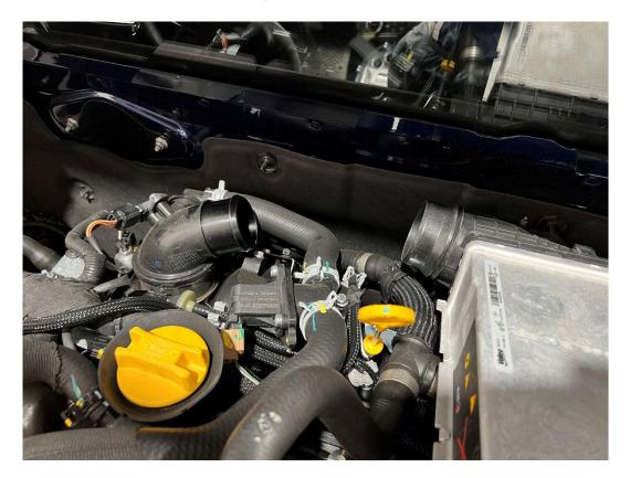
8. Remove the breather hose to the turbo inlet.
