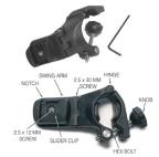
notch in the slider clip to the rear. Swing the hinge down to make contact with the handlebar. Swing the hex bolt up, seating the knob into its recess. Turn the knob clockwise to tighten and secure the mount to the handlebar.
