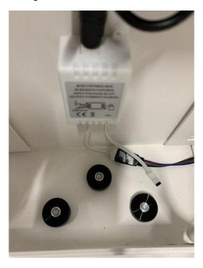
Next, secure the top piece bracket to the top of pedestal using the three (3) thumb screws.
