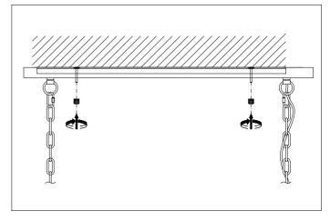
4. Place the canopy over the ceiling plate fix it with the nuts.
