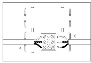
**3.** Connect the 3 wires according to their colours. Brown is the live wire (L), blue is the neutral wire (N), green/yellow is the earth wire ( $\frac{\bot}{-}$ ).
