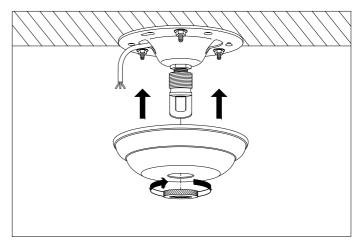
2. Slide the canopy over the ceiling plate and fix the retaining nut.
