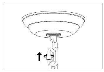
3. Hang the lamp from the suspension eye, using the chain and carabiner. Carefully lower the lamp until the chain is taut. Straighten the chain links.
