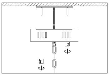
**3.** Carefully place the canopy over the ceiling plate and fix the canopy with the nuts provided.
