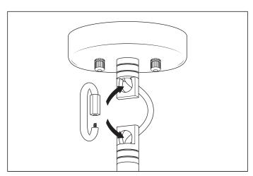
5. Link the lamp to the canopy using the chain link. Securely close the chain link once the lamp is linked to the canopy.
