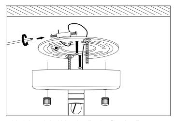
**4.** Lock the steel wire tightly to the ceiling plate. Place the ceiling canopy over the ceiling plate and fix it with the nuts.
