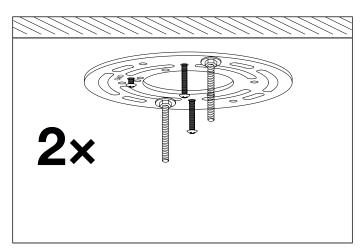
Fix the crossbar to the ceiling by using mounting plugs and screws suitable to your ceiling type.
