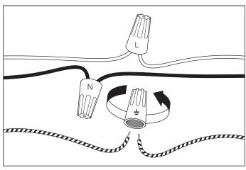
**3.** Connect the 3 wires. L is the live wire, N is the neutral wire. The course wire is the grounding wire.
