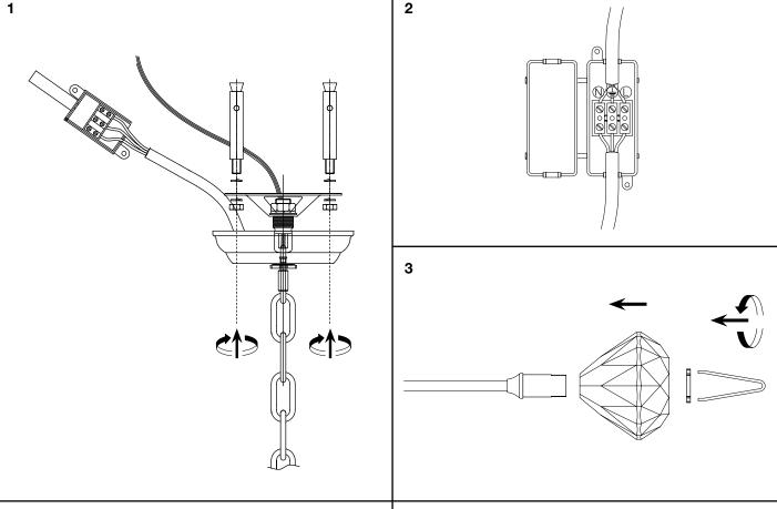
Turn-off the electricity supply at main circuit panel before installing. Do not connect electricity supply until your ceiling light is fully assembled and installed.
