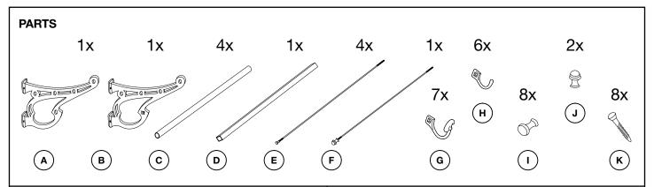
**1** Put left bracket A and the right bracket B on the floor standing on their base. Insert square pipe D loaded with hooks G and hangers H to the square slots in both the brackets.
