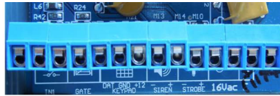
Low Voltage Terminal
