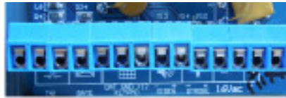
Low Voltage Terminal
