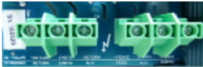
High Voltage Terminal
