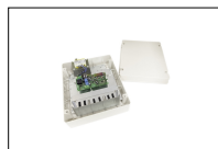
B71/PBX36/BOX Hybrid inverter, "Network Assisted" version, for powering the automation. Also provides a battery-charger function thanks to the connection to the solar panels or mains supply for powering the 36V DC brushless digital controllers with a mains voltage of 230V AC.
