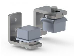
Rebate bearing hinges fit inside the frame of the gate to achieve a clean minimalist finish with very low post to gate gaps. They are the ideal hinge for automated aluminium driveway gates. The bottom hinge features a tapered thrust bearing and the top hing has a sealed ball bearing.
